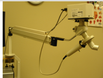
Figure 2: The mouthpiece to measure IOS attached to the loudspeaker
